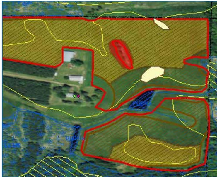
**Maps like this one are used to record the many details biosolids operators keep track of in the field, such as setbacks from waterways, wetlands and drinking water wells. The computer data are loaded on a Global Positioning Device mounted in the operator's tractor for precise work in the field.**
