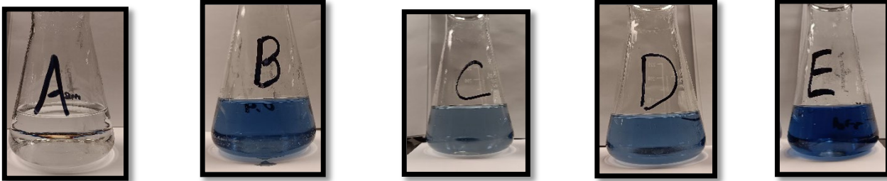
Figure 3. Images of wastewater samples after chemical reaction to test for phosphorus has occurred.
